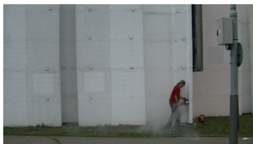
Fig. A1. Taking samples from a noise barrier treated with FN2 two years earlier, on a sunny day without rain for at least 7 days before.
